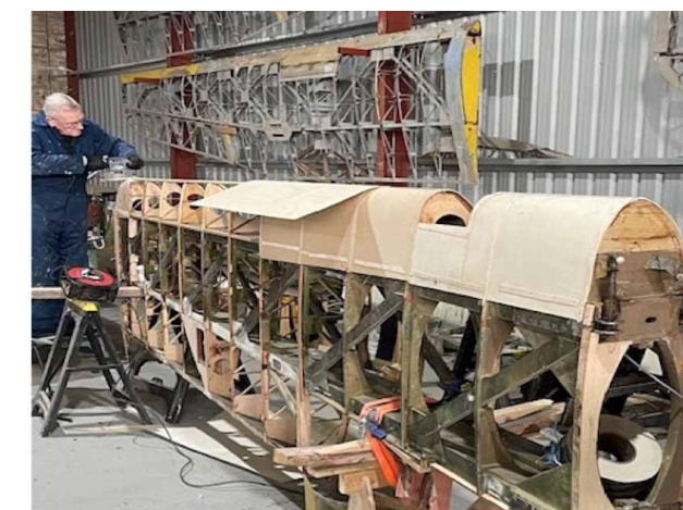
Percival Proctor wing rebuild.
