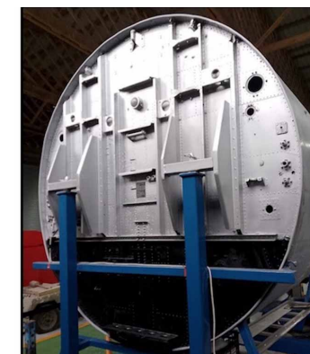
Rear bulkhead tidied, repainted and made safe.
