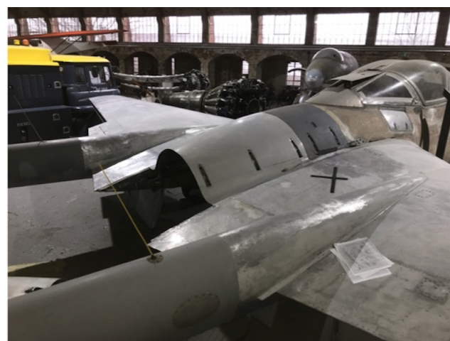
Two cowls in place.
