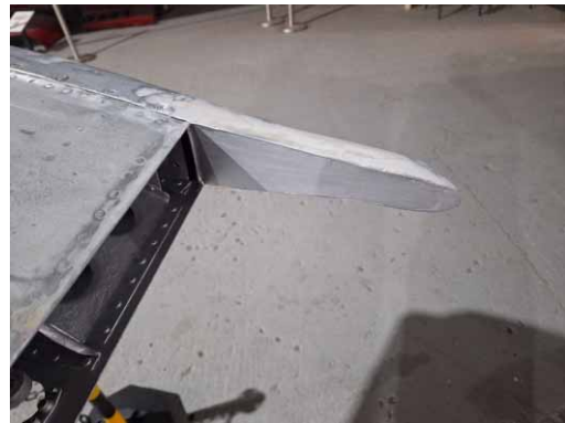
Starboard wing tip repaired.
