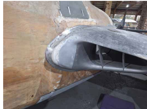
Port wing nose repaired and wing/fuselage fairing fitted.
