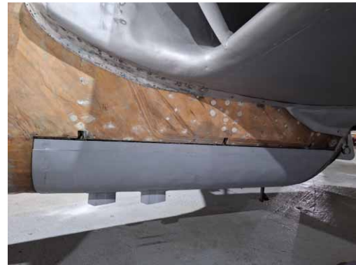
Port side, gun compartment door fitted.
