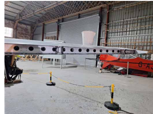
Starboard wing aileron recess prepared.
